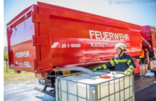
Ablassen in IBC-Container
